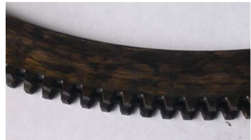
Fig. 9. Traces of the damage on a steel disc after tests
