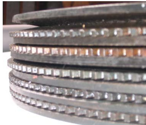
Fig. 8. Deformed package of discs of brake F_5 after tests
