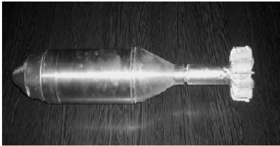
Fig. 7. Steel model with tail and nose FDM and Chromium coating
