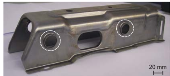
Fig. 1. The need for movable system inside the forming tool to produce necks outwards
