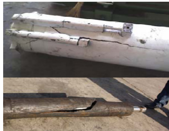
Fig. 1. The damaged hydraulic cylinders
