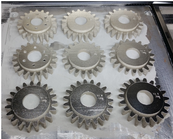
Fig. 1. A set of gears on the building platform after the melting process using the DMLS method
