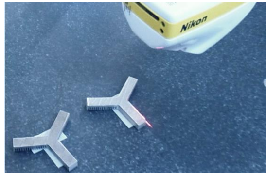
Fig. 6. Part measurement with non-contact laser scanner.
