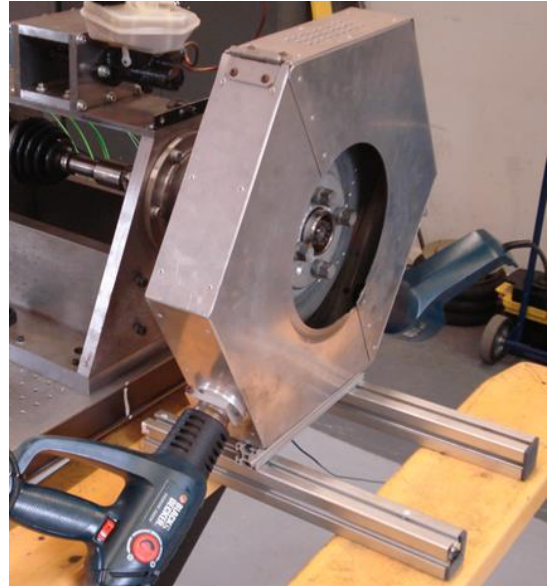
Fig. 3b. Thermal Spin Rig - heating box
