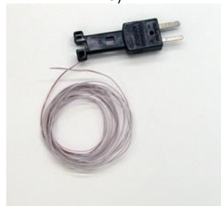
Fig. 4. Thermocouples used: (a) Rubbing/Contact thermocouple and (b) Wire thermocouple
