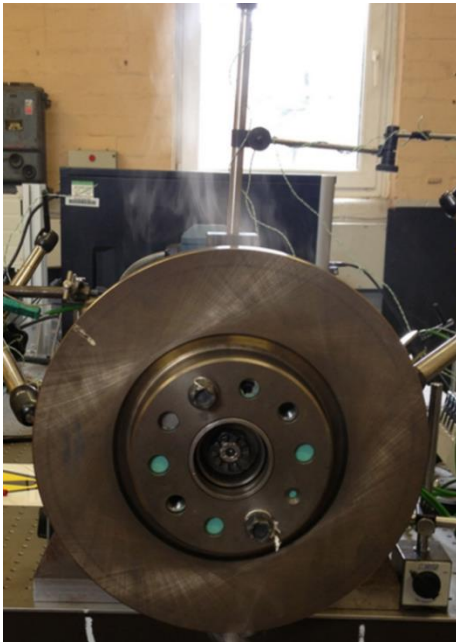
Fig. 10b. Ventilated disc: flow (smoke) pattern using smoke generator
