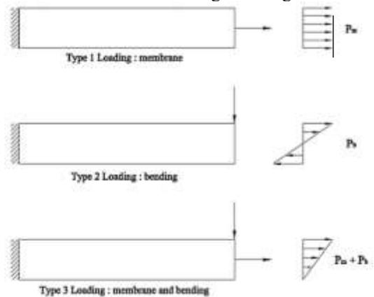
**Fig. 10.** Types of loading on butt weld joint
