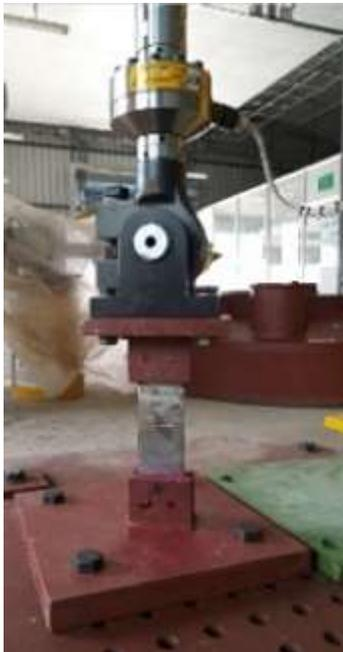
Fig. 11. Butt joint under fatigue loading
