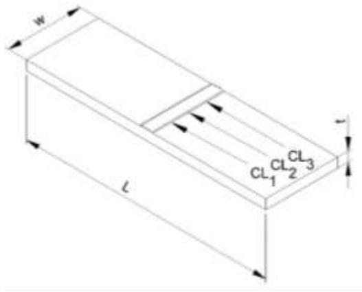
Fig. 1. Crack locations in butt welded joint
