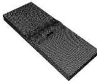
**Fig. 8.** Finite element model of butt joint
