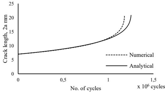
**Fig. 6.** Comparison of crack propagation life of a cruciform joint
