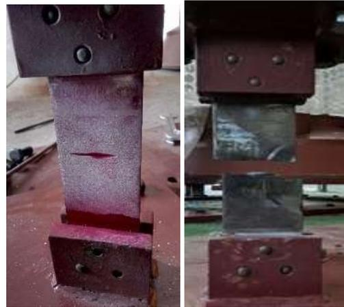
a) Initial notch b) Fractured specimen
