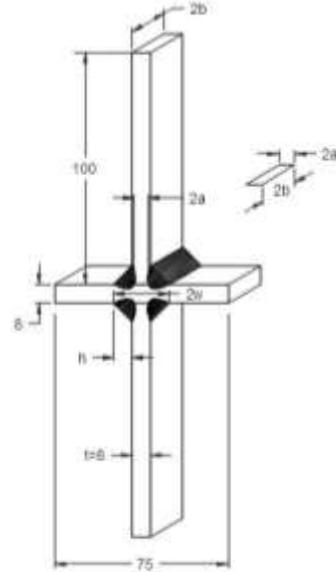
Fig. 2. Cruciform joint with LOP defect
