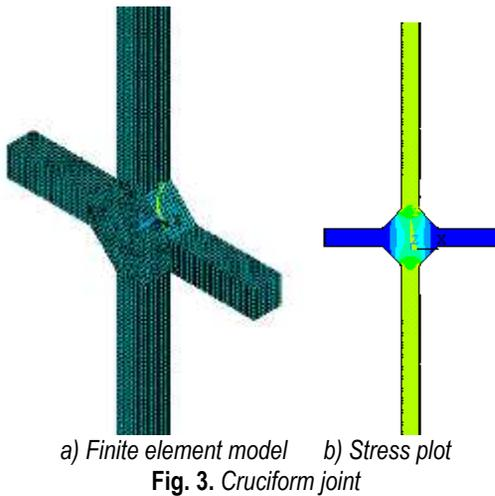
After performing stress analysis using Ansys software, the finite element model along with nodal displacements is imported into Franc3D software. A double edge crack of length  $2a = 7$  mm
