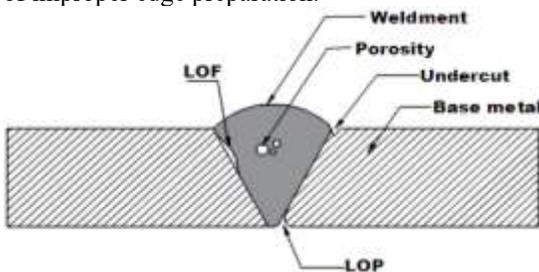
**Fig. 7.** Types of weld defect
