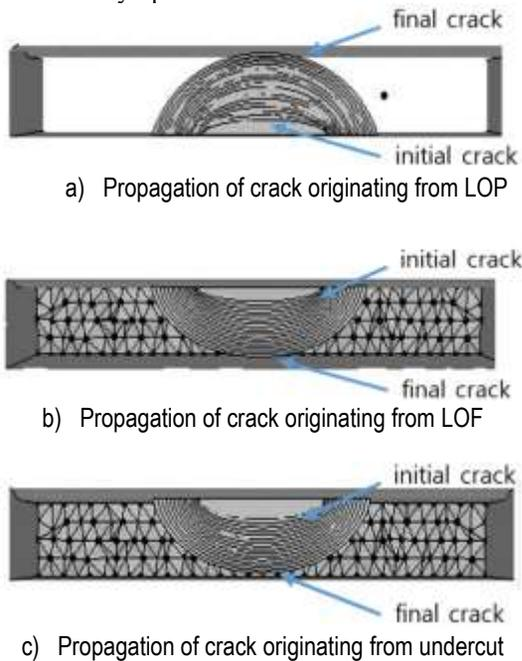
**Fig. 9.** Numerical simulation of crack propagation in butt weld joint
