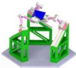
Fig. 11. Structural configuration of the 3-CRU PM when TMI=1 and CCI=1
