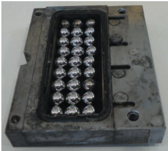
Fig. 6. Mould slot filled with bearing balls
