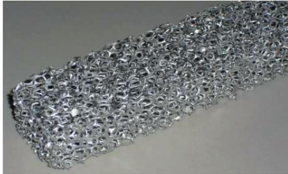
Fig. 5. Insert made of open cell aluminium foam
