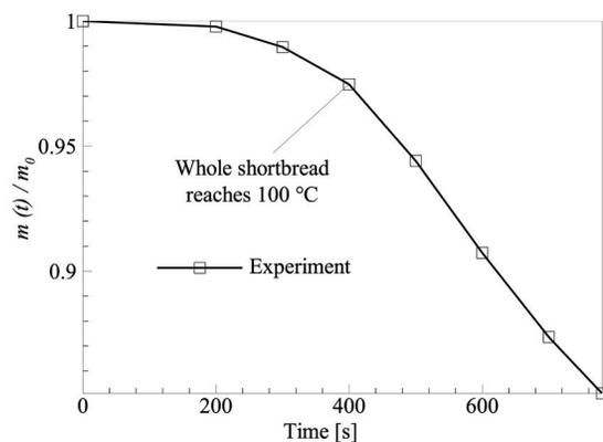
Fig. 4. Shortbread mass change due to the evaporation of the water; the mass at the start of the baking process was  $m_0$  and the mass as a function of time during the baking process was  $m(t)$
