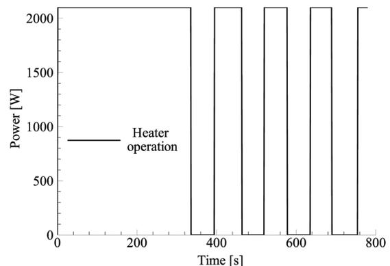
Fig. 2. The operation of the round heating element during the baking process
