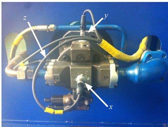
Fig. 1. Installation of the vibration sensors
