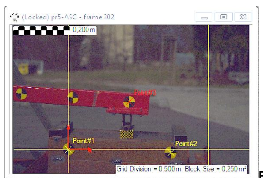
ig. 4. The moment of ram impact – frame by TEMA Motion
