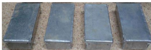
Fig. 5. The steel containers filled with iron-based porous materials compositions.
