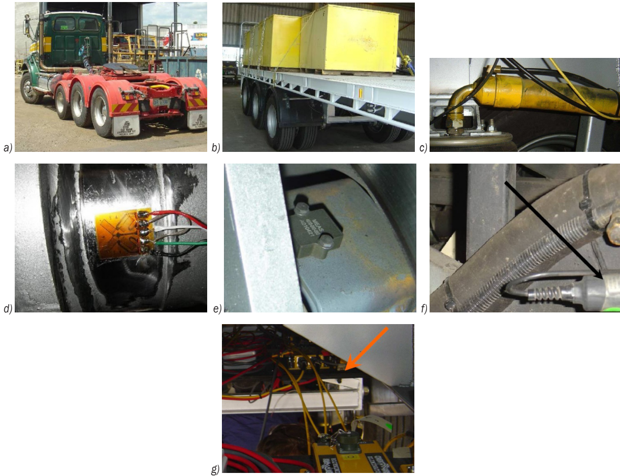
Fig. 2. Setups of the tests; a) prime mover, b) test semi-trailer with test load, c) large longitudinal air line, d) strain gauge, e) accelerometer mounted on the axle, f) air pressure transducer, g) CHEK-WAY telemetry system underneath the semi-trailer [26]
