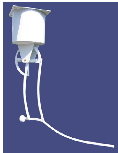
Fig. 3. Manufactured aluminium mechanism used for kinematic tests
