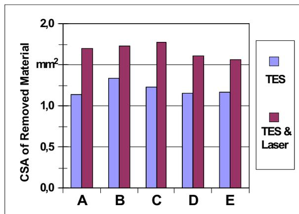
Fig. 1. Cross-sectional area (CSA) of the removed material by dry-ice blasting and laser-assisted dry-ice blasting
