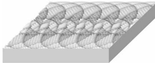
Fig. 4. *3D profile plot, rotating head with swivelling*
