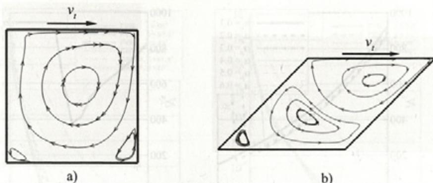
Fig. 2. Streamlines in laminar flow in a lid-driven cavity a)  $\beta = 90^\circ$ , b)  $\beta = 45^\circ$
