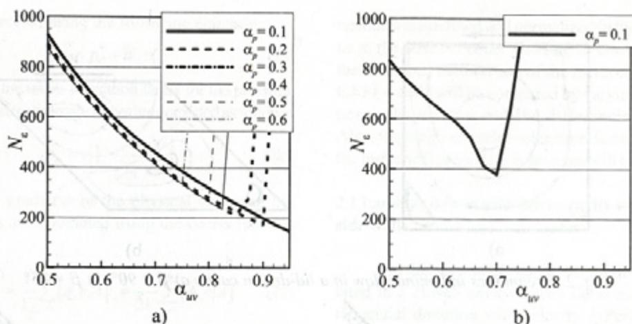
Fig. 5. Number of outer iterations required to reduce the residual levels to  $\epsilon = 10^{-6}$  for the lid-driven cavity problem for  $\beta = 45^\circ$  (UDS) a) FVM, b) CAFFA
