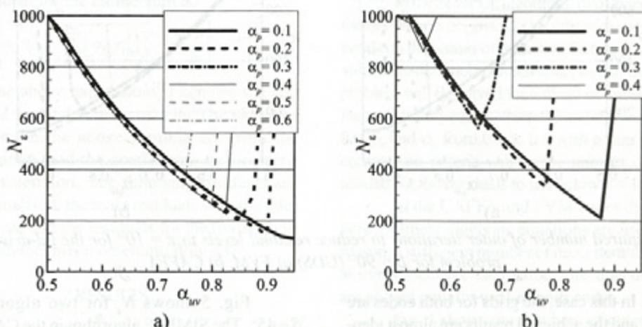
Fig. 6. Number of outer iterations required to reduce the residual levels to  $\epsilon = 10^{-6}$  for the lid-driven cavity problem for  $\beta = 67.5^\circ$  (UDS) a) FVM, b) CAFFA
