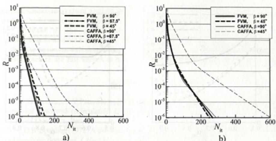
Fig. 7. Convergence histories for the SIMPLE algorithm in the FVM and CAFFA codes for the lid-driven cavity problems a) UDS, b) CDS scheme
