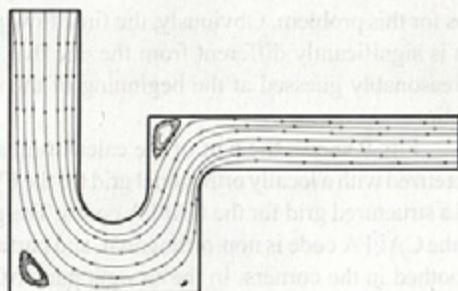
Fig. 8. Streamlines for laminar flow in a curved channel
