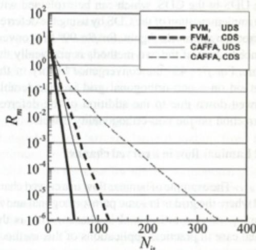
Fig. 11. Convergence histories for the SIMPLE algorithm in the FVM and CAFFA codes for the curved-channel problem (UDS and CDS)
