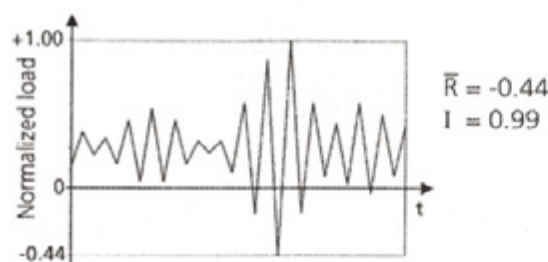
Fig. 10. Test spectrum of cast aluminium rear axle steering rods
