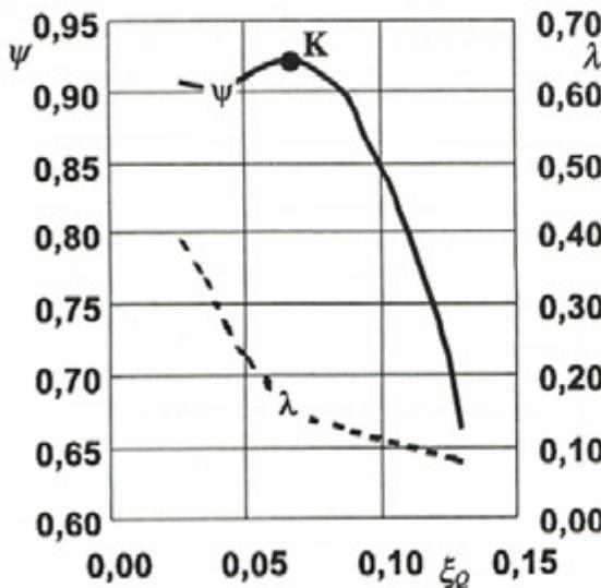
Sl. 3. Obratovalna karakteristika ( $\xi_Q$ - $\psi$ ) in ( $\xi_Q$ - $\eta$ ), dodan sekundarni tokFig. 3. Capacity-Head ( $\xi_Q$ - $\psi$ ) and Capacity-Efficiency curve ( $\xi_Q$ - $\eta$ ), added secondary flow
