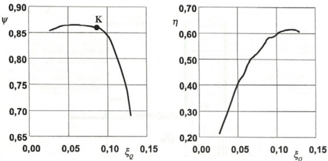
Sl. 2. Obratovalna karakteristika ( $\xi_Q$ - $\psi$ ) in ( $\xi_Q$ - $\eta$ )Fig. 2. Capacity-Head ( $\xi_Q$ - $\psi$ ) and Capacity-Efficiency curve ( $\xi_Q$ - $\eta$ )
