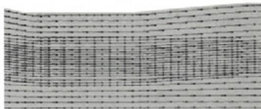
Fig. 13. Velocity field at 100% opening of guard-gate
