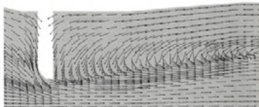
Fig. 11. Velocity field at 30% opening of guard-gate
