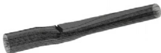
Fig. 9. Streamlines at 70% opening of guard-gate
