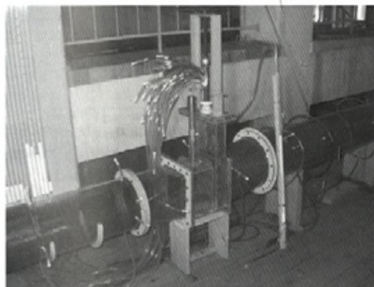
Fig. 14. Model of the pressure tunnel; gate chamber with gate, hoist mechanism, piezometric taps and aeration pipe; and penstock
