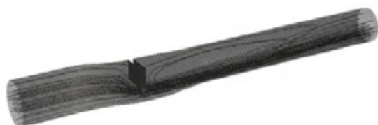
Fig. 8. Streamlines at 30% opening of guard-gate
