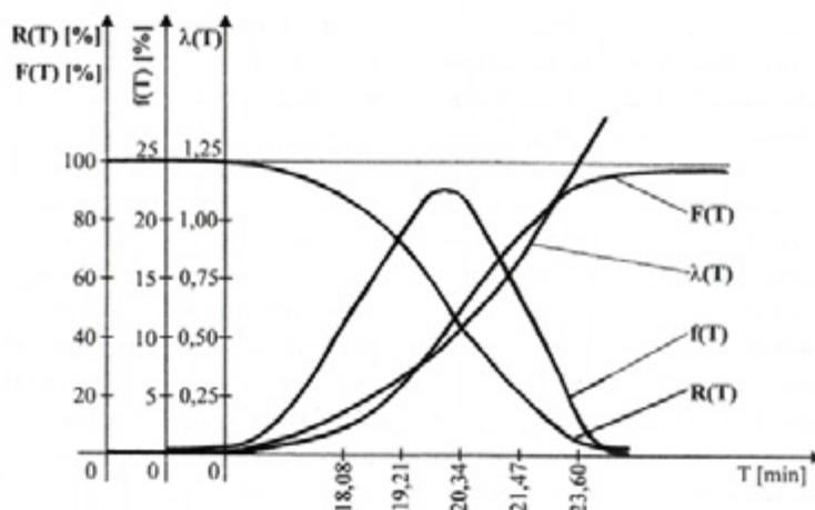
Fig. 3. Graphic presentation of main indicators for the normal model of reliability of CBN cutting tools in turning of 20CrMo5 steel
