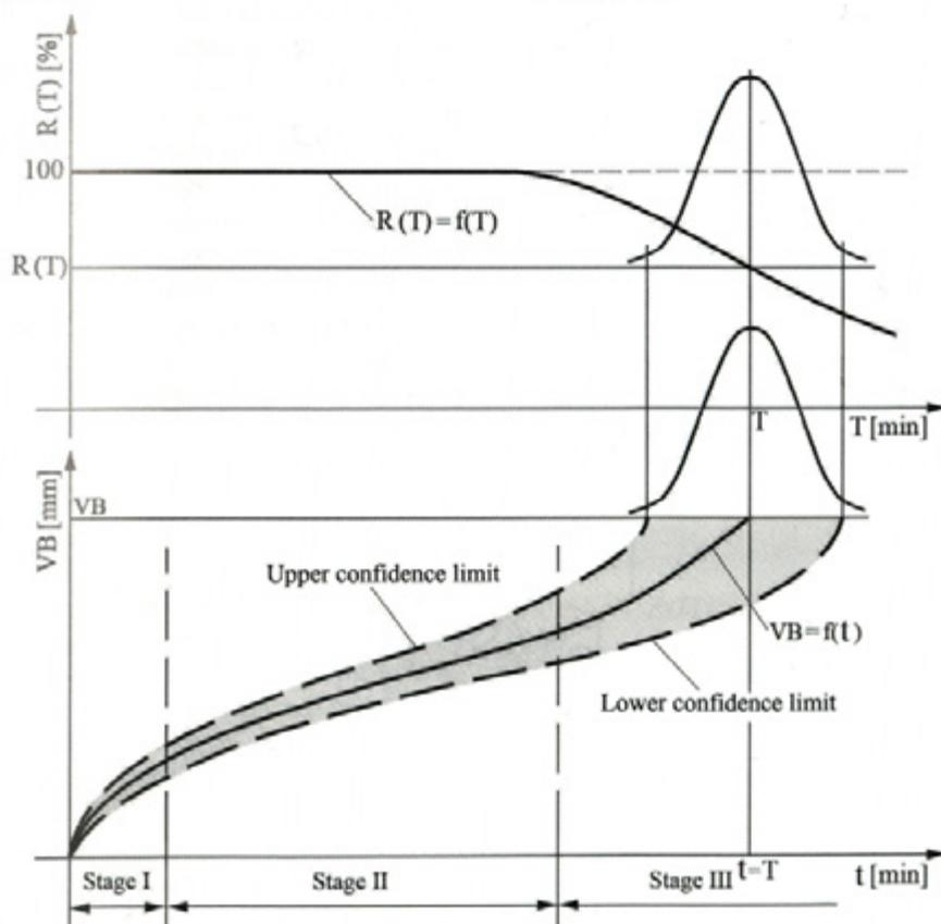
Fig. 1. Graphical illustration of the interaction between tool wear and reliability within a tool cycle
