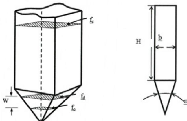
Fig. 5. Harrow tooth modulation - Wear effects
