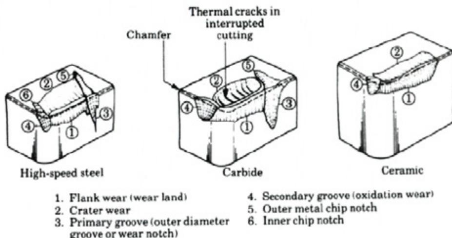
Fig. 2. Tool wear mechanisms for different tool materials [26]
