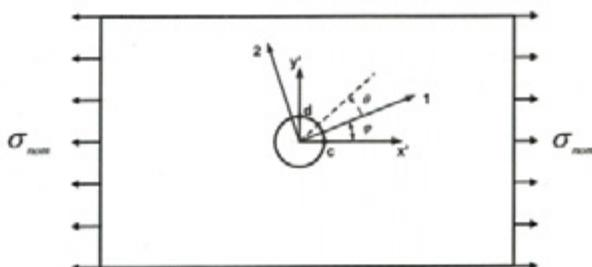
Fig. 2. An infinite-plate containing a central circular opening
