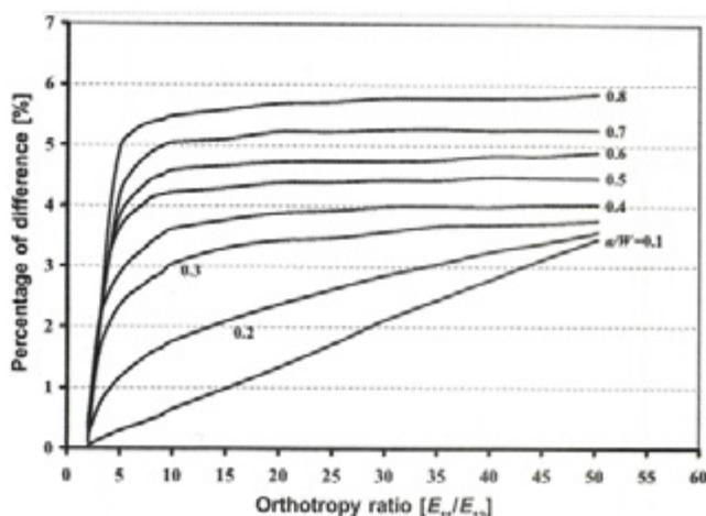
Fig. 8. Difference of analytic and FE method results
