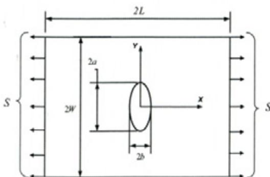
Fig. 1. A finite-width plate containing a central elliptical opening
