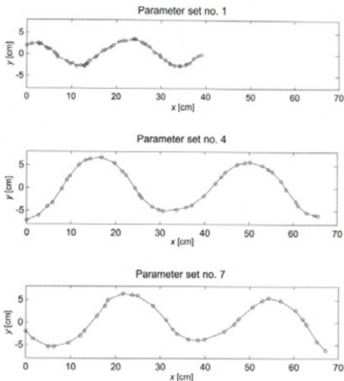
Fig. 10. Head trajectories measured at different combinations of control parameters. At parameter combination 7, the robot achieved the highest velocity.
