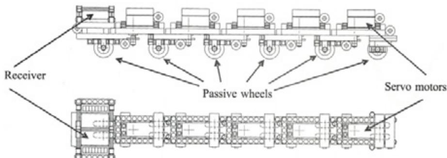
Fig. 5. Drawing of a complete experimental snake-like robot
