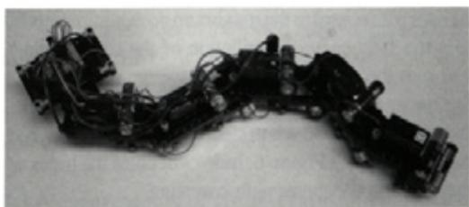
Fig. 4. Final version of a snake-like robot
