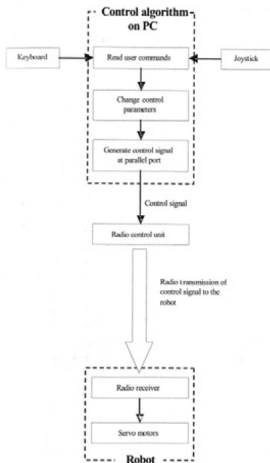
Fig. 7. Flow diagram of control system
