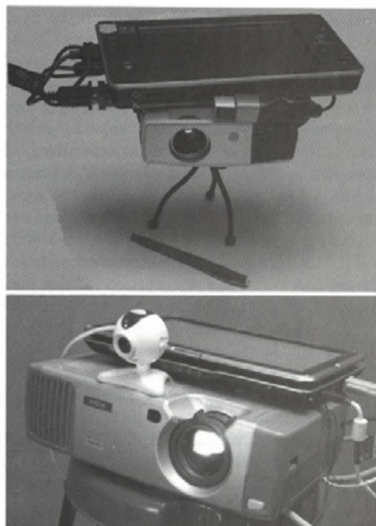
Fig. 2. Pilot versions of I/O Pads: handheld (top) and large (bottom) I/O Pads
