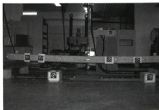
Fig. 3. Prefabricated prestressed concrete plate with measured marks
