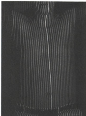
Figure 3: The image of the volunteer's frontal torso illuminated by the laser multiple-line projector
