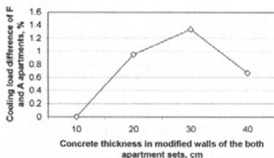
Fig. 9 Difference of cooling loads for the thermally non-insulated apartments with F and A-walls as given a function of thickness of modified concrete.
