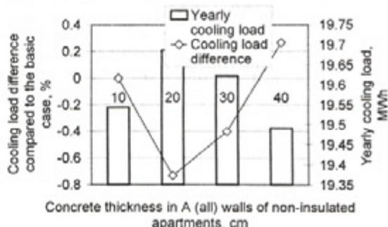
Fig. 8. Cooling load and its difference as functions of thickness of concrete in thermally non-insulated A-walls. The difference is compared to the basic case.
