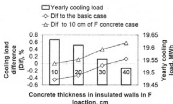
Fig. 5. Cooling load and cooling load difference as functions of thickness of concrete in insulated F-walls. The difference is given for cooling loads compared to a) the basic case, and b) thermally insulated F case with 10 cm of concrete. Here, modified walls have 5 cm of thermal insulation.
