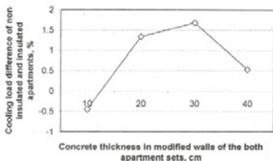
Fig. 6. Difference of yearly cooling loads for thermally non-insulated and insulated apartments. This difference is given as a function of thickness of concrete in F-walls.
