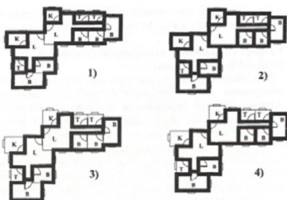
Fig.3 Envelope and partitions arrangements: 1) E arrangement, 2) A arrangement, 3) T arrangement, and 4) U arrangement where B stands for bedroom, L for living and dining room, K for kitchen, and T for toilet.
