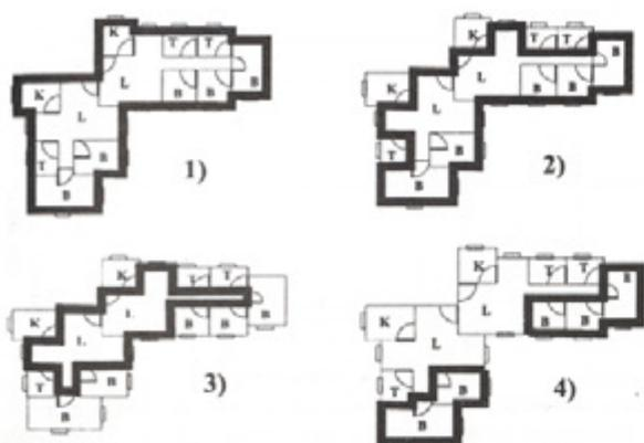
Fig.2 Envelope and partitions arrangements: 1) F arrangement, 2) W arrangement, 3) L arrangement, and 4) D arrangement where B stands for bedroom, L for living and dining room, K for kitchen, and T for toilet.
