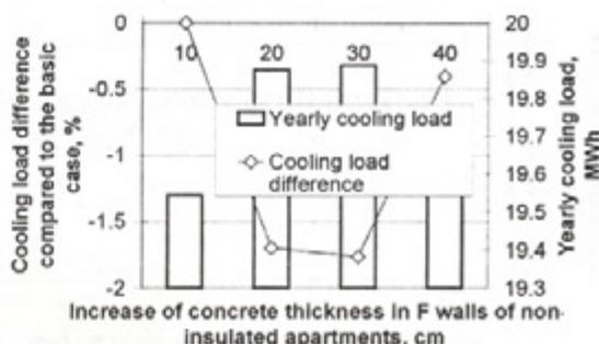
Fig. 7 Cooling load and its difference as functions of thickness of concrete in thermally non-insulated F-walls. The difference is compared to the basic case.
