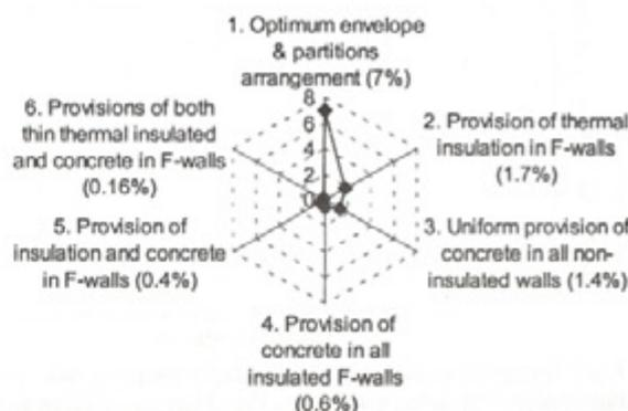
Fig. 10 The radar list of the minimum values of cooling load recorded in different investigations.
