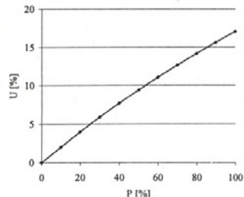
Figure 2 – Energy savings in the production of packaging glass using crushed glass
