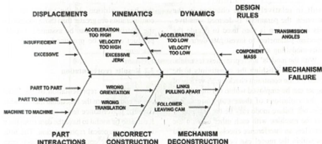
Fig. 2. Ishikawa diagram of system failures
