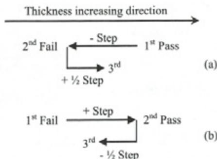
Fig. 5. Situations involving “ $\pm \frac{1}{2}$  Step” of thickness change: (a) “+  $\frac{1}{2}$  Step”; (b) “-  $\frac{1}{2}$  Step”
