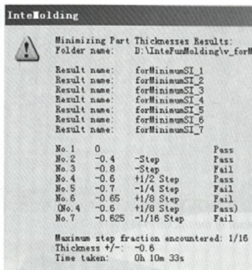
Fig. 13. Thickness-minimization results when multiple molding-quality criteria are used
