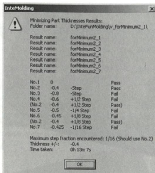
Fig. 7. Thickness-minimization results for the studied design case
