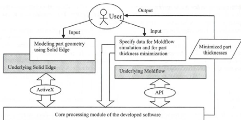
Fig. 2. System framework of the developed software
