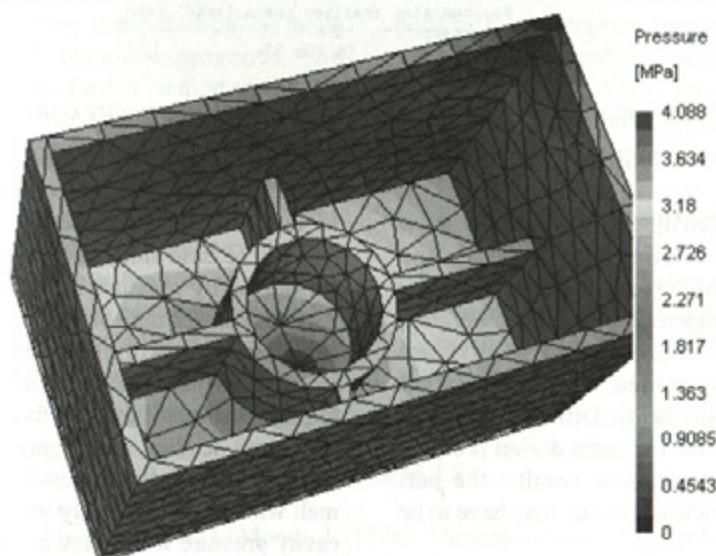
Fig. 12. Pressure distribution after the changed molding-quality criteria
