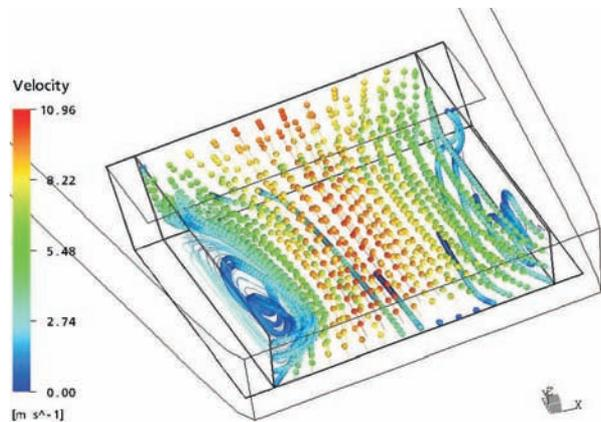
Figure 9: Streaklines in the inner part of the heater.
