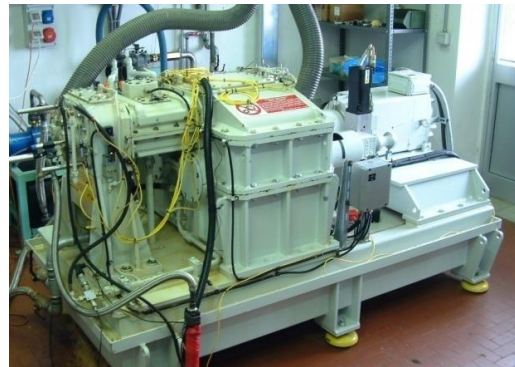
Fig. 4. Test rig for the characterization of aerospace gears
