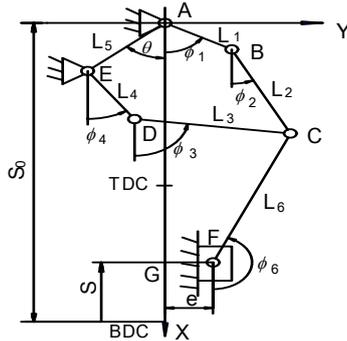
Fig. 1. Sketch of hybrid-driven press
