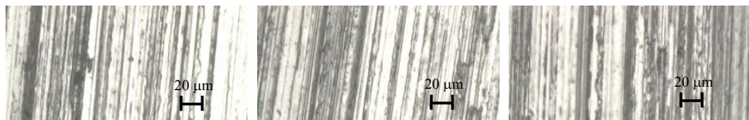
a) Depth of cut: 0.01 mm b) Depth of cut: 0.02 mm c) Depth of cut: 0.03 mm Fig. 7. The influence of depth of cut on surface structure for the grinding wheel of 60 grain
