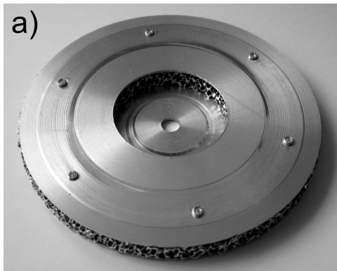
Fig. 2. a) Bladeless impeller without and b) bladeless impeller with radial inducer
