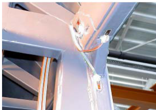
Fig. 2. Adherence of the measuring tapes
