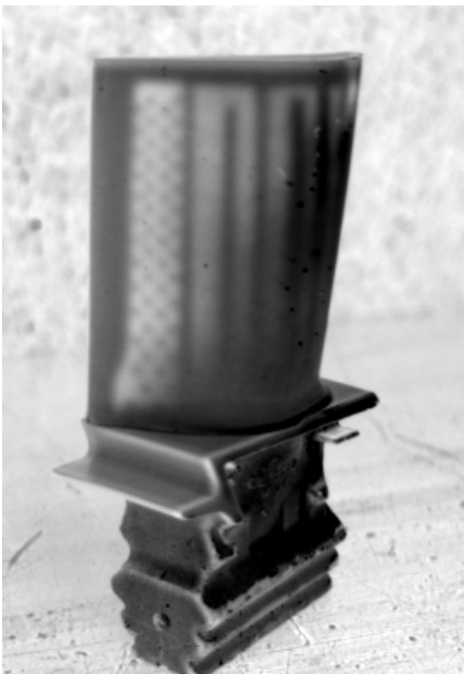
Fig. 4. Cooling channels of a turbine blade, imaged with optically excited Lockin-Thermography (lockin frequency 1 Hz)
