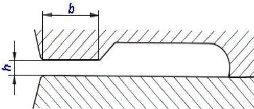
Fig. 2. Dimensions of flash land of forging dies
