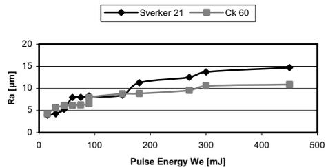
Fig. 2. Variation of average roughness  $R_a$ , with pulse energy,  $W_e$
