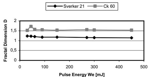
Fig. 14. Variation of fractal dimension  $D$  with pulse energy,  $W_e$
