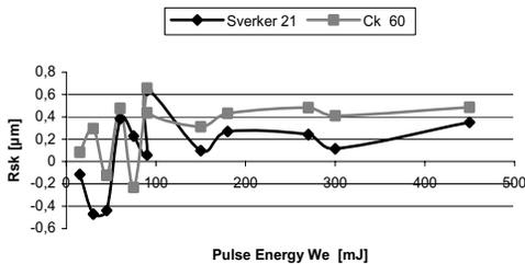
Fig. 3. Skewness of the heights distribution  $R_{sk}$ , versus pulse energy,  $W_e$
