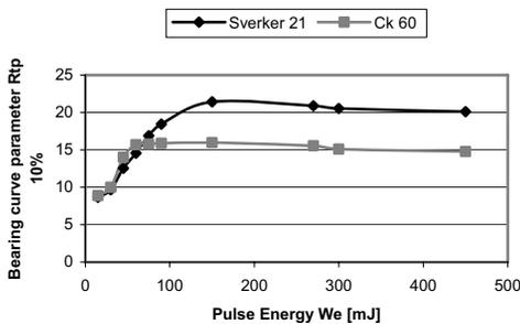
Fig. 7. Variation of  $R_{tp10\%}$  parameter of roughness profile with pulse energy,  $W_e$
