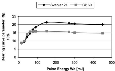
Fig. 7. Variation of  $R_{tp10\%}$  parameter of roughness profile with pulse energy,  $W_e$
