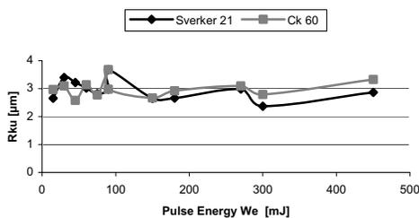
Fig. 4. Kurtosis of the heights distribution  $R_{ku}$  versus pulse energy,  $W_e$
