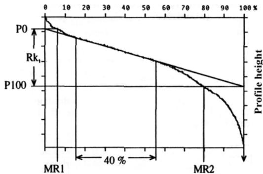
Fig. 1. Definition of the family of " $R_k$ " parameters
