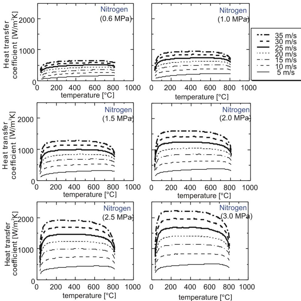
Fig. 4. Example of heat transfer coefficients in gas quenching (nitrogen gas)
