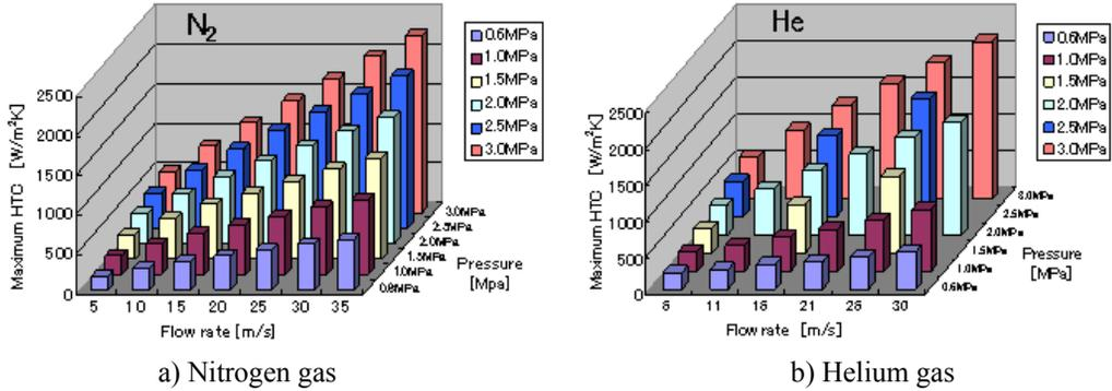
Fig. 5. Effect of flow rate and pressure on maximum heat transfer coefficient in gas quenching
