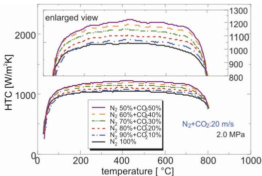
Fig. 8. Effect of mixing rate of carbon dioxide gas on heat transfer coefficient in nitrogen and carbon dioxide mixture gas cooling (2.0 MPa, 20 m/s)
