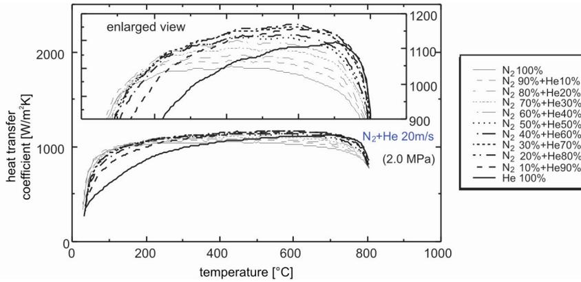
Fig. 6. Effect of mixing rate on heat transfer coefficient in nitrogen-helium mixture gas cooling (2.0 MPa, 20 m/s)
