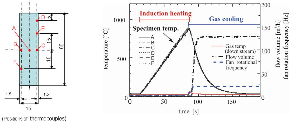
Fig. 3. An example of measured data in heating and gas cooling of silver probe
