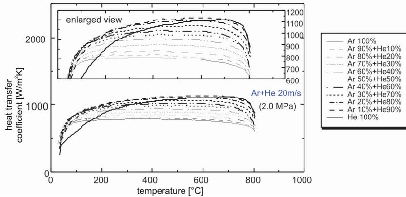
Fig. 7. Effect of mixing rate on heat transfer coefficient in argon-helium mixture gas cooling (2.0 MPa, 20 m/s).
