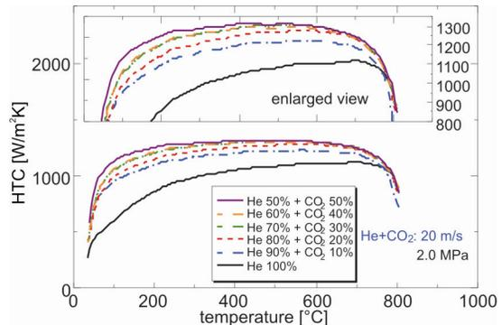
Fig. 9. Effect of mixing rate of carbon dioxide gas on heat transfer coefficient in helium and carbon dioxide mixture gas cooling (2.0 MPa, 20 m/s)
