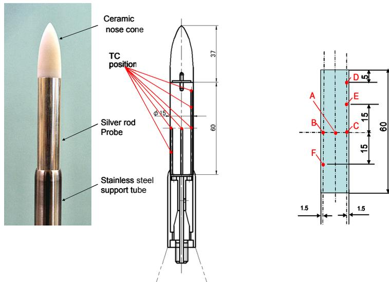
Fig. 1. Silver rod probe and positions of thermocouples
