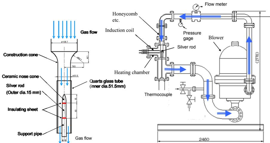
Fig. 2. Gas-quenching test apparatus
