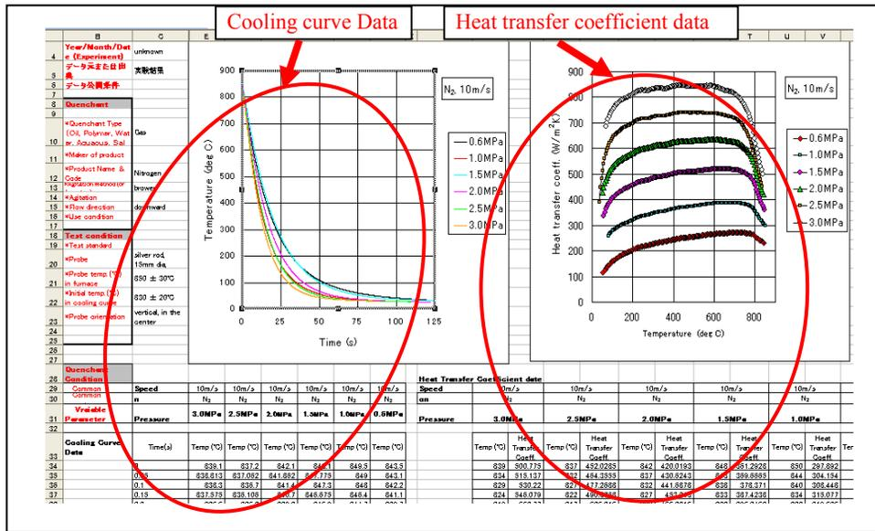
Fig. 10. An example of data sheet in database of cooling power of quenchants
