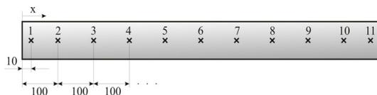
Fig. 6. Measuring-position placement on the analyzed beam
