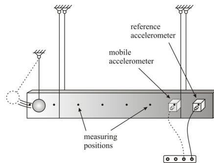
Fig. 7. The validation-experiment configuration set-up
