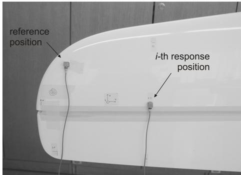
Fig. 11. A horizontal tail with accelerometers placed at the reference position (left) and at the *i*-th response position (right)
