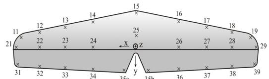
Fig. 10. Measuring positions' placement and the global coordinate system of the horizontal tail
