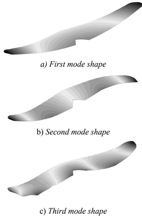
Fig. 12. Reconstructed normalized horizontal tail's mode shapes
