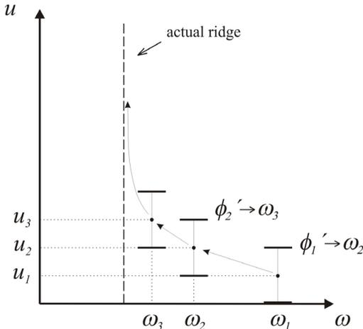
Fig. 2. Ridge detection using the phase method with the recursive equation (14)
