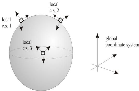
Fig. 5. Problem of spatial vibration measurements
