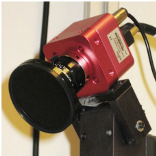
Fig. 1. 1 Megapixel camera with IR filter
