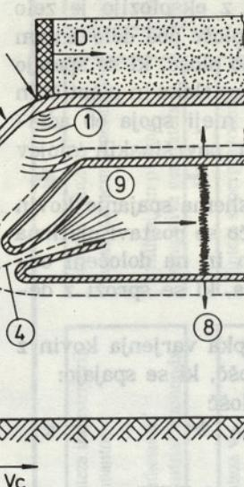
The collision takes place successively, along the base plate at velocity  $v_p$ . The collision with the base material results in a very high pressure (around 1 Mbar). The collision point travels along the plate at velocity  $v_c$ . Under the influence of »surface« cumulative flow, oxides, and other impurities on the two surfaces are decomposed, and partly removed from the bonding area.
