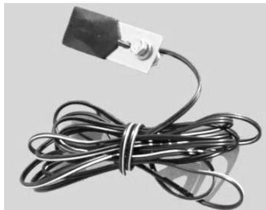
Sl. 2. Magnet in rele za merjenje vrtilne frekvence kolesa Fig. 2 Magnet and the reed-relay used for sensing the rotation of the wheel
