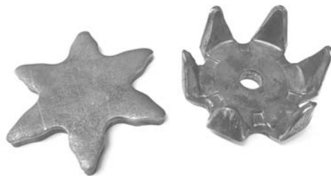
Sl. 1. Platina in izdelani krempljasti pol alternatorja Fig. 1. Blank and finished claw pole for alternators
