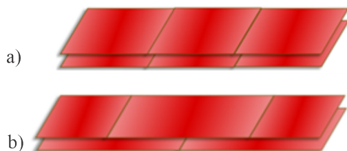
Fig. 4. Schematic diagram of the scanning mode of processing grid superposition; a) repeated scanning of a single grid, and b) cross-stacked scanning of A-B grid
