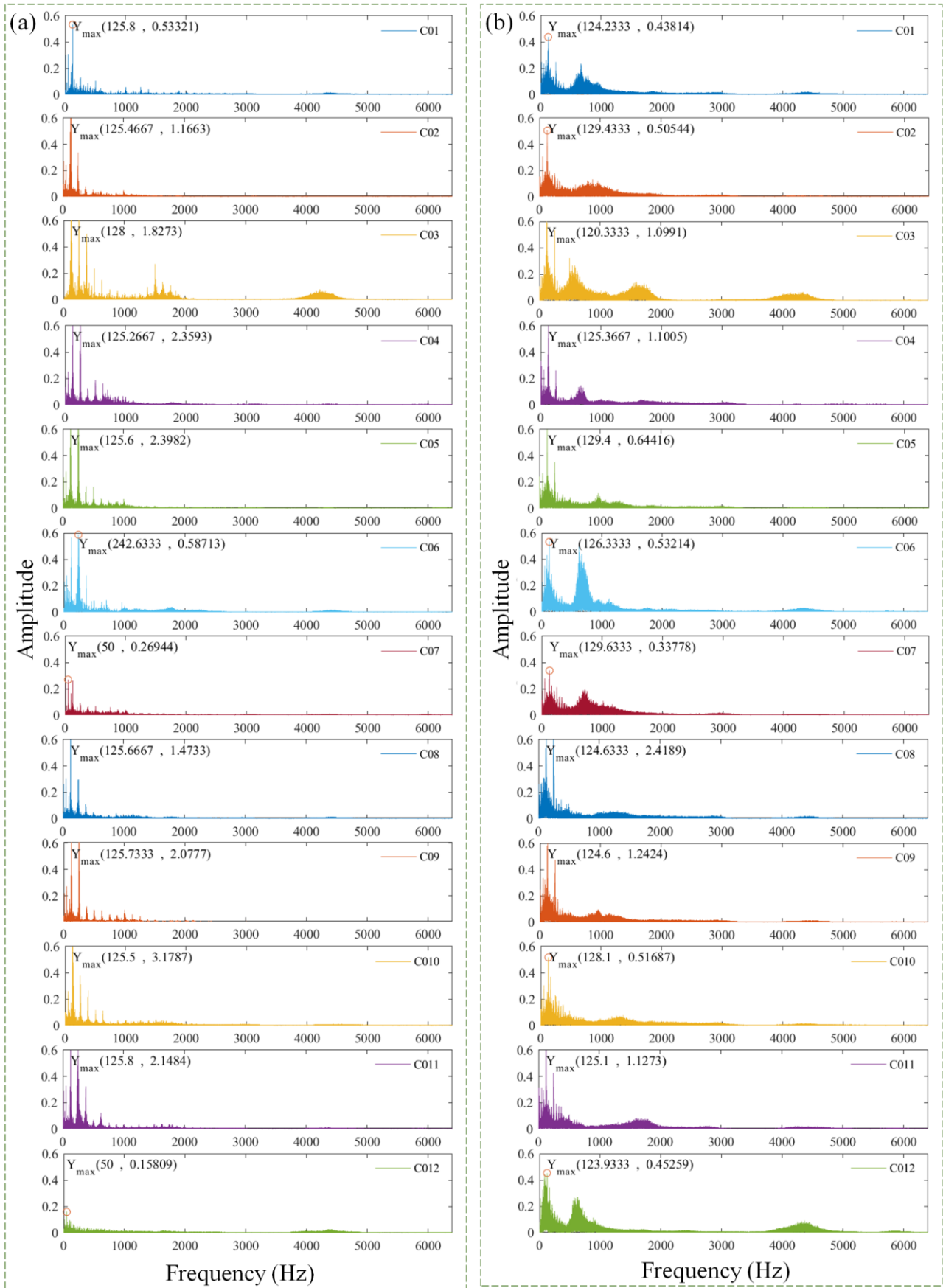
Fig. S4: Representative frequency-domain vibration signals of different groups in the Y-axis/ Normal direction at: (a) the 1800 th s; (b) the 16200 th s.
