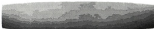
Fig. 11. Visualization of D_k on casting E_4. (light: +0.04 mm above R_p ; dark: -0.04 mm below R_p )
