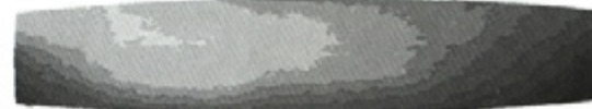
Fig. 9. Visualization of D_1 on casting E_2. (light: +0.7 mm above R_k , dark: -0.7 mm below R_k )
