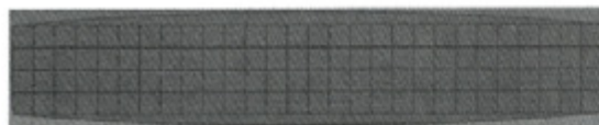
Fig. 8. ROI 1 divided to a matrix of 28 x 4 segments whose average size is 5 x 5 mm
