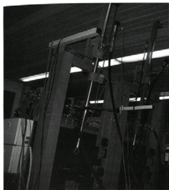
Fig. 6. Water (on the left) and oil (on the right) hydraulic cylinder with load masses
