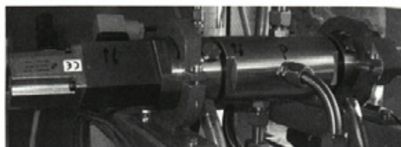
Fig. 4. The specimen – prototype of the proportional 4/3 directional control valve for water hydraulic
